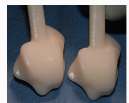
Figure 9: The two trial implants made from medical grade plastics
